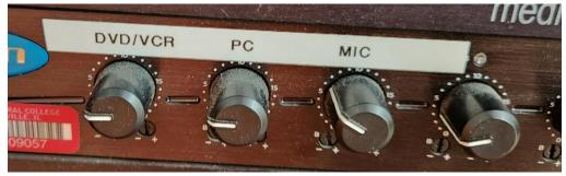
The knob on the left of the mixer labeled **PC** adjusts the volume of the computer audio.
